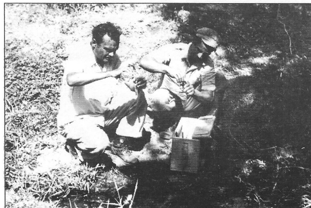
37. Determinando la concentración de componente químico en el agua (Uso del colorímetro) [Determining the concentration of chemical component in the water (use of the colorimeter)]. — Haskins colorimetric field test for sodium pentachlorophenate. Mateo on the left.
